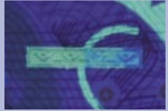
left-hand part of blind code fluoresces green, right-hand part fluoresces blue (green fluorescent element described below)
